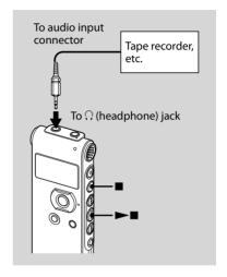
To record the sound of the IC recorder with other equipment, connect the  $\Omega$  (headphone) jack of the IC recorder to the audio input connector (minijack, stereo) of other equipment using an audio connecting cable\*.
